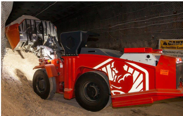
WIPP's first all-electric vehicle, a load-haul-dump, is already working in the underground. Its batteries are recharged from an underground power station.
